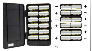
I. Close cover of DCell BBU and ensure that cover "snaps" and is securely fastened.
