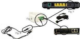
C. Connect "Y" Cable [Fig. 2] to the DCell BBU Input Port [Fig. 6] using the "Y" Cable Input Connector [Fig. 8]
